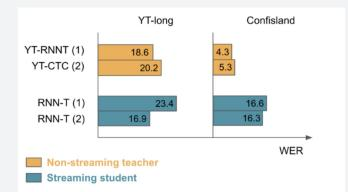
Figure 4: Comparing a RNN-T streaming student model trained from CTC and RNN-T non-streaming teachers. The CTC model is a better teacher, despite having a higher WER.
