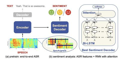
**Fig. 1**. We propose to use pre-trained features from e2e ASR model to solve sentiment analysis. The best performed sentiment decoder is RNN with self-attention. We apply SpecAugment to reduce overfitting in the training.
