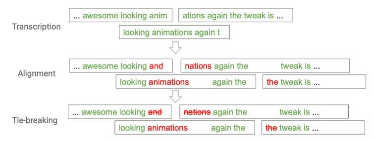
**Fig. 2**: Overlapping inference. The algorithm first breaks a long utterance into overlapped segments, each of which is then transcribed independently. It then merges the transcripts from overlapped segments into a consensus transcript for the original long utterance. In case there are conflicts in predictions, it prefers the predictions further from the utterance boundary.
