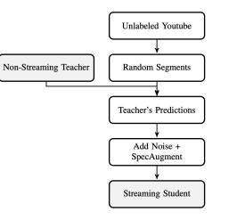
**Fig. 1.** Our method trains a streaming model, learning from the predictions of a powerful non-streaming teacher model on large-scale unlabeled data via a teacher-student training framework. See Sect. 2.2 for more details.
